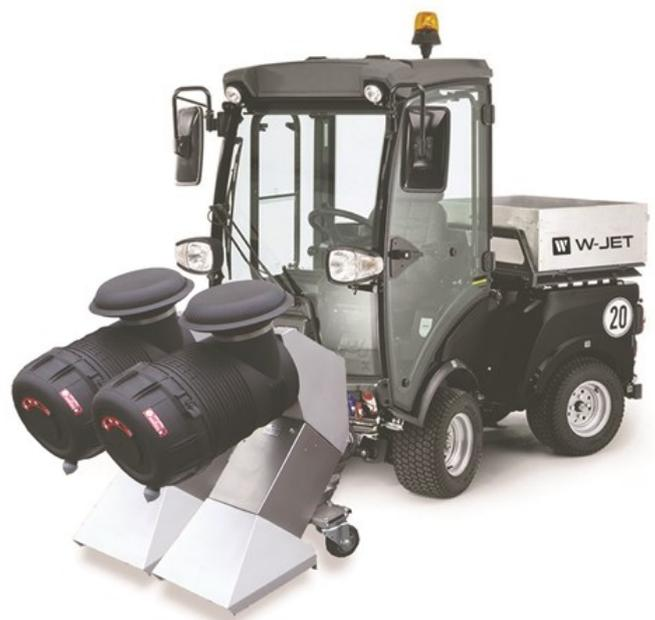
The M1 module can be adapted on any suitable carrier.
